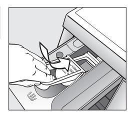
■ If you are using liquid detergent, use the liquid detergent insert in the main wash compartment Ш.
